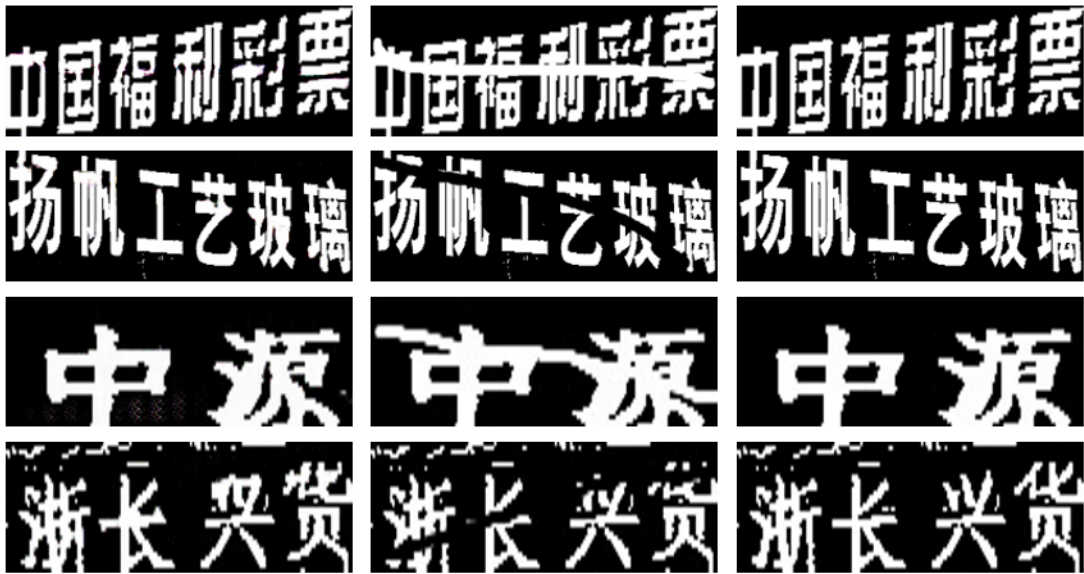
Fig. 7. The result of Pix2pix. On the left column are restored images, in the middle column are blocked images, and on the right column are real images.
